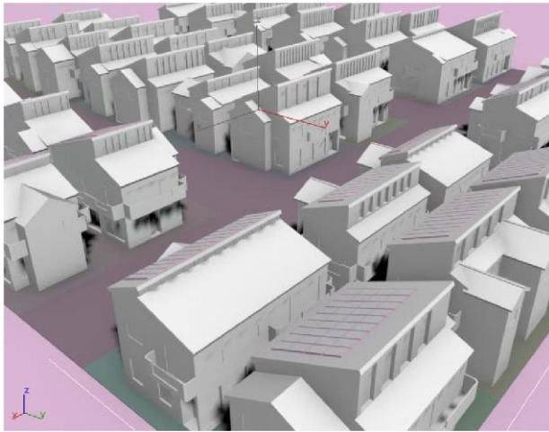
Figure 7. 3D building models with double leaned roof automatically generated after land readjustment
