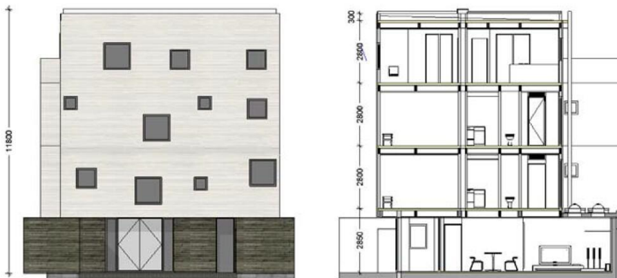
Figure 3. Elevation and section views of the building that are automatically generated by Allplan
